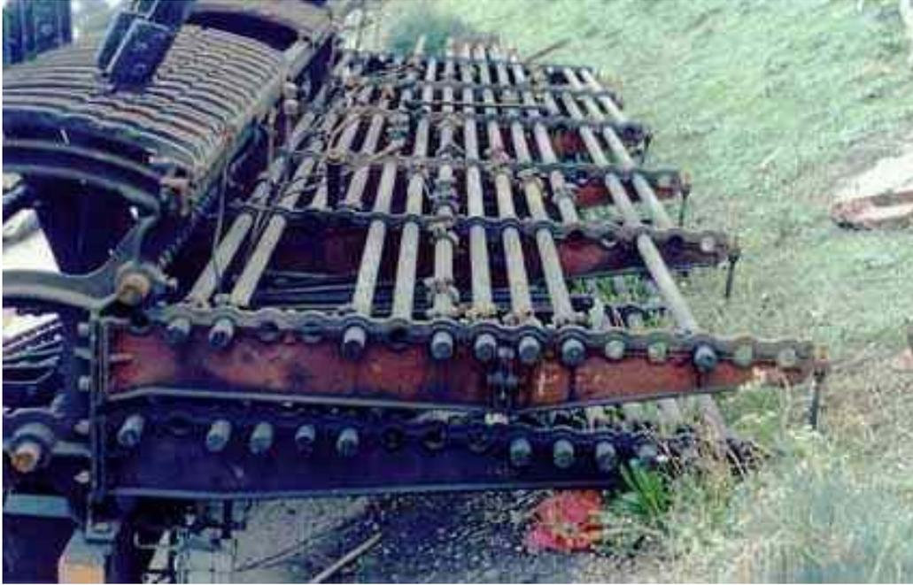
**A view of the rocking shaft brackets from the left hand end of the frame. Two tiers of rocking shafts can be applied to a frame (known as the `top' and `bottom' rocking shafts). Thirty shafts could be fitted to the Newport A frame; 15 in the top bracket (which has 16 holes, but the first could not be used as it fouls the cam tails) and 15 in the bottom bracket.**
