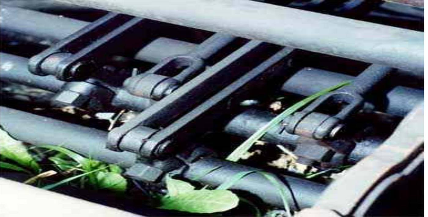
**A detail shot of the soldiers clamped to two rocking shafts. The lower shaft has the drive from a cam; the cam links are the two flat parallel mild steel bars (1 1/2" by 5/16"), one placed each side of the soldier head. The upper rocking shaft has a drive from a cam at left, and locks on the two adjacent levers. Lock rods are solid 3/4" wrought iron rods with a forged eye to connect to the soldier head. Each lock rod is different, and must be made to order by a blacksmith.**
